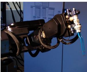
There aren't many instruments that can be used in conjunction with an MRI, all because of that pesky M. Standard metal objects get pulled away by the strong magnets that produce the image, and anything that produces a magnetic field itself distorts the picture. So most of the robot is made of titanium or a plastic composite. That's where Johnson Medtech comes in.
