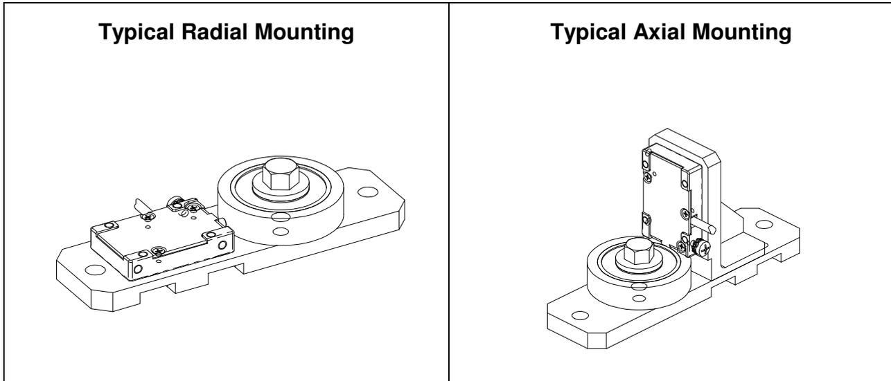
In general, while performance is comparable, axial mounting is more forgiving of concentricity errors in the bearing structure and the finger tip maintains a flat contact pattern. Mounting in a radial manner will cause the finger tip to take a slightly curved shape during the conditioning process.
