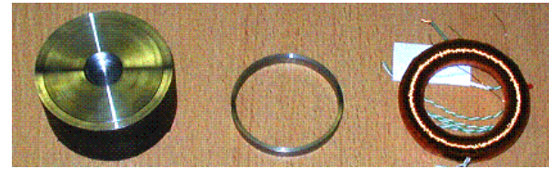
Preparation of raw material UGITECH 416, machining in the form of torus and winding
