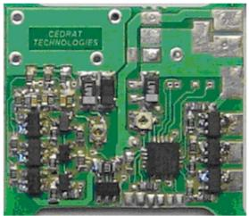
Figure 5 : View of the BLDC control board
