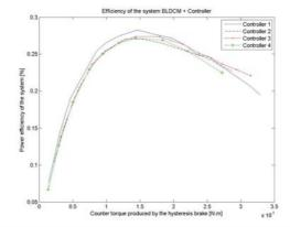
Figure 7: Comparison of the efficiency of the motor + drive electronic
