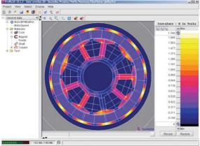
Figure 3: Flux modelling of the BLDC
