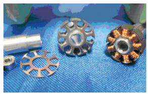
Figure 1: View of the BLDC parts
