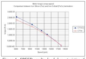
Figure 4 : SPEED results: load characteristics of the BLDC
