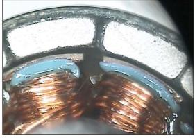
Figure 2: Detailed view of the air gap
