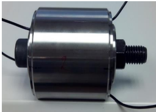
Figure 16: The ultrasonic transducer for radial excitation assembly
