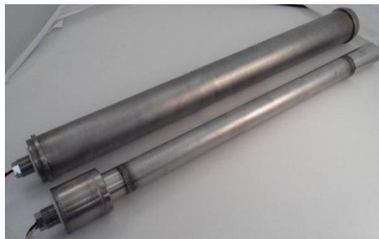
Figure 18: The MUST and conventional ultrasonic tube transducer
