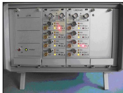
Figure 10. Picture of a rack with two LWDS45-2 modules, i.e. multi-channel drive and sense electronic for piezo-patches.
