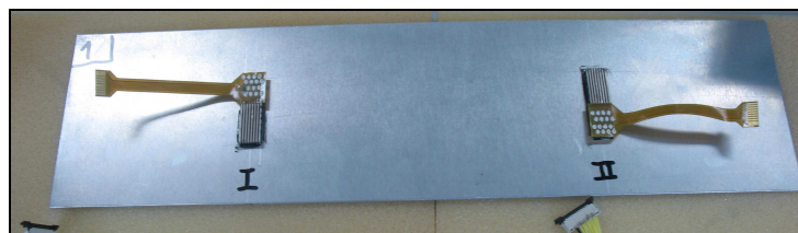
Figure 8. Picture of an aluminium test plate with integrated piezo-composite patches.
