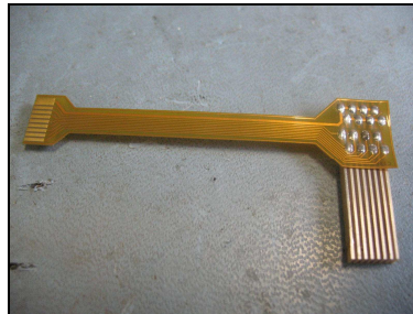
Figure 7. Integration of the flex PCB on a piezo-composite sample.
