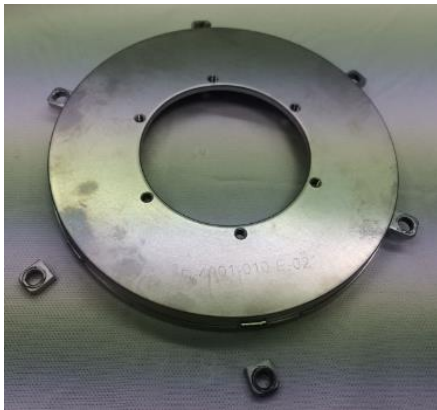
Figure 7: Two legs broken
