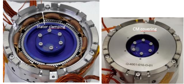
Figure 8: On QM model, one part for stator clamping and another for CM covering
