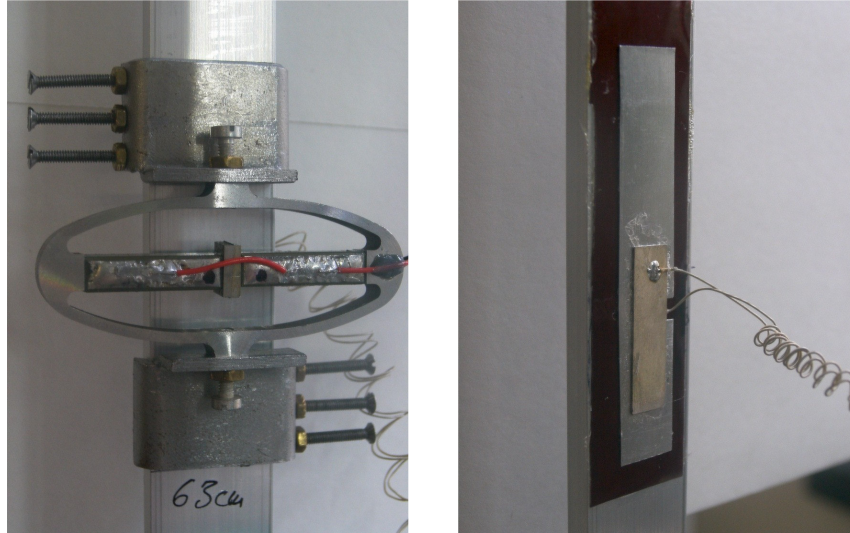
Figure 4.1 Actuator and sensor mounted on the beam
