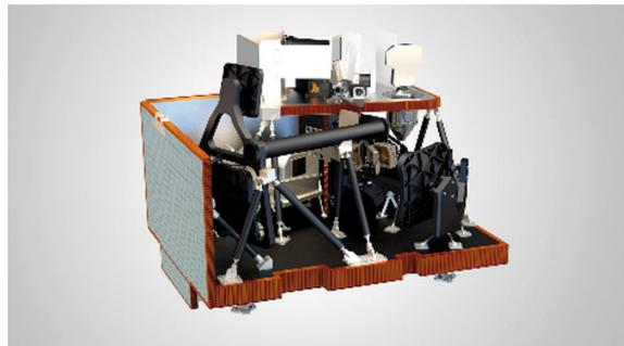
**Fig. 7:** IASI-NG instrument (courtesy of AIRBUS DS)
