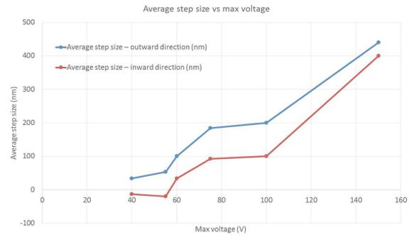
**Fig. 5:** Average step size vs supply signal max voltage
