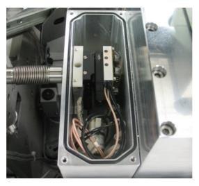
Fig.6: FPS200M on a XY stage on a MX Beamline (Courtesy ESRF)
