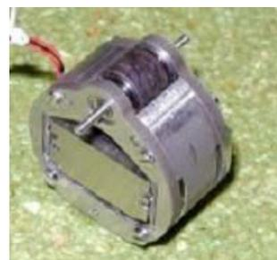
Fig. 6: Small rotary motor – type RPM60
