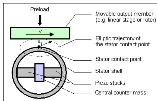
Fig. 1: UPD-based motor concept
