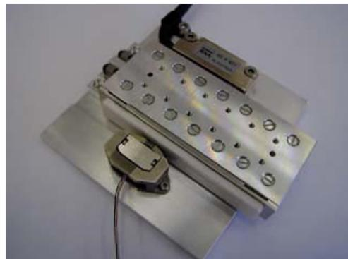
Fig. 5: UPD60 drive unit actuating a linear stage
