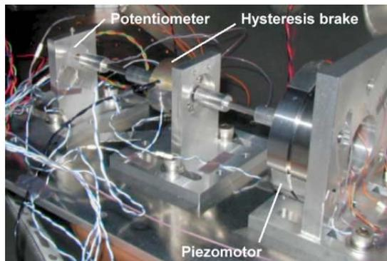
Fig. 10: Instrumented test rig inside the vacuum chamber
