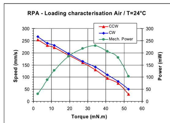
Fig. 9: Initial loading characterisation of the motor
