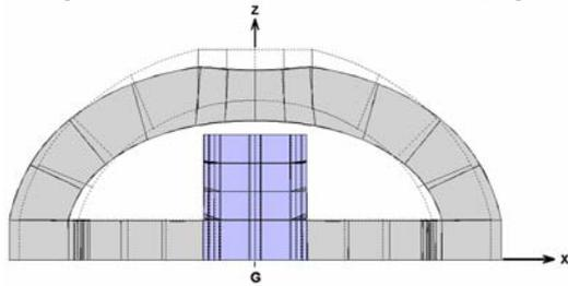
Fig. 2: FEM simulation of the flexural mode
