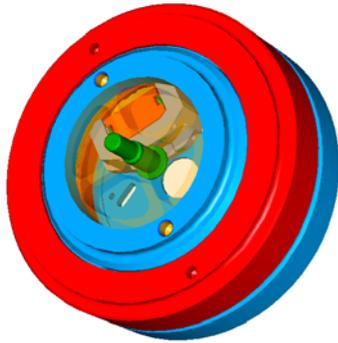
Fig. 7: Rotary motor configuration with visible internal UPD unit (top cover not shown)
