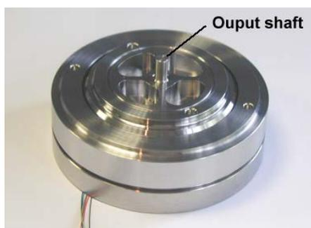
Fig. 8: Rotary motor prototype (RPA)
