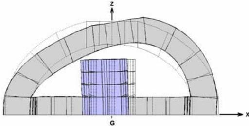
Fig. 3: FEM simulation of the translation mode
