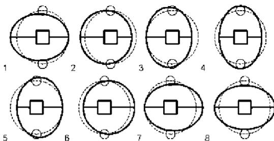
Fig. 4: Basic motion sequence of the vibrating stator
