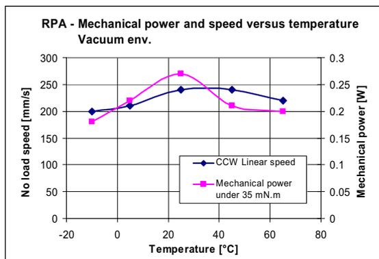
Fig. 11: Motor performances in vacuum (thermal cycling)
