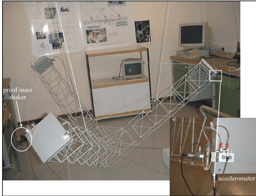
Space truss from ULB, integrating an active control of vibrations based on tendons actuated by APA100Ms
