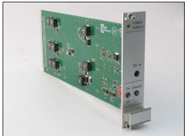
Figure 3.2 Power supply for the generation of magnetic field.
