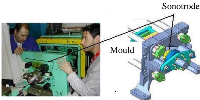
This part has been made with the new moulding machine using ultrasound. It is 2 mm in diameter. A new mould has been developed especially adapted to the ultrasound requirements. The second figure shows the part enveloped in a feeding ring that is slightly different from conventional mould tapping systems.
